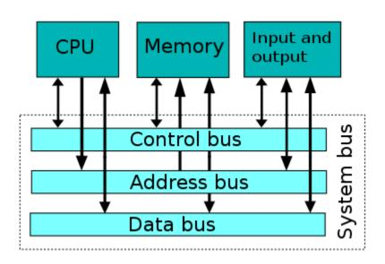
**BUS:** In computing, a bus is defined as a set of physical connections (Cables, Printed circuits, etc.), which can be shared by multiple hardware components in order to communicate with one another.
